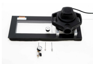
VACUUM BOX TEST POLYWELD Y LEISTER
